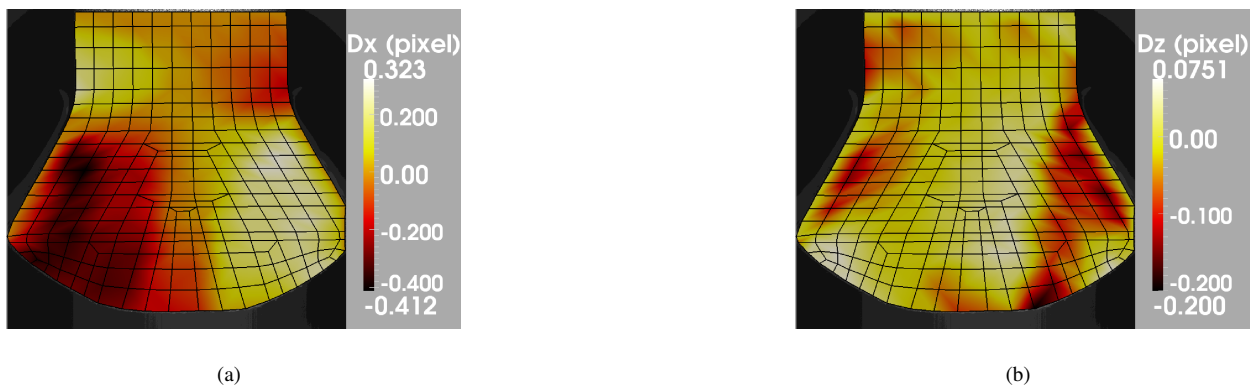
Figure 16: Local displacement residual ( i.e. , difference \mathbf{u}_m - \mathbf{u}_c ) projected onto (a) the x -axis, and (b) the z -axis. Units are in pixel
