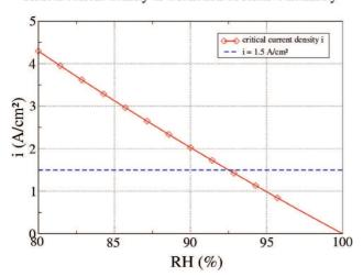
Fig. 2 — Critical current density  $i_{\text{c}}$  as a function of relative humidity RH in the channel.
