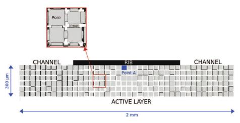
Fig. 1 - Sketch of GDL as a two-dimensional pore network.
