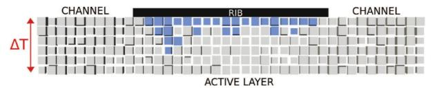
Fig. 5 – Partial liquid invasion of the GDL by condensation under the rib. Each little square corresponds to a pore. Liquid phase in blue, gas phase in grey. Pattern obtained for RH = 97% (channel);  $i = 1.5 \text{ A/cm}^2$ ;  $\Delta T = 3.25 \text{ K}$ . (For interpretation of the references to color in this figure legend, the reader is referred to the web version of this article.)
