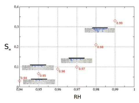
Fig. 7 – Variation of overall water saturation as a function of a channel relative humidity RH for  $i = 1.5 \text{ A/cm}^2$  together with corresponding condensation invasion patterns (for RH = 0.94, 0.95, 0.97 and 0.99 respectively). Each little square corresponds to a pore. Liquid phase in blue, gas phase in grey.  $\Delta T = 3.25 \text{ K}$ . (For interpretation of the references to color in this figure legend, the reader is referred to the web version of this article.)
