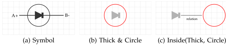
Fig. 12. An example showing use of spatial relation in the context of symbol recognition. To make it simple, we use spatial predicate (inside, a topological relation) to define the connectivity between the pair of primitives: thick (or filled component) and circle that compose a symbol.
