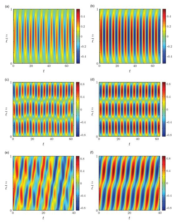
**Fig. 3.** Cross-flow displacement of the tensioned cable predicted by DNS (left) and by the model (right):  $\ell$ =0.55 and  $\xi$ =3.65 in (a) and (b),  $\ell$ =1.50 and  $\xi$ =3.65 in (c) and (d),  $\ell$ =1.00 and  $\xi$ =0.04 in (e) and (f).
