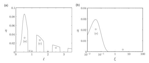
**Fig. 4.** Left: evolution of the efficiency with the reduced length  $\ell$  for  $\xi$ =3.65; right: evolution of the efficiency with the damping parameter  $\xi$  for  $\ell$ =1. Model results (solid lines) and DNS results (symbols). The letters (a), (c) and (e) correspond to the DNS results shown in Fig. 3.
