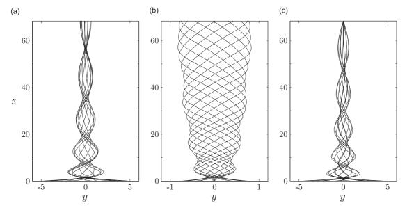
**Fig. 10.** Selected instantaneous positions of a hanging cable VIV with a damped upper extremity for  $\ell = \ell_{opt}$  and three different damping parameters : (a)  $\xi = \xi_{opt}/100$ , (b)  $\xi = \xi_{opt}$  and (c)  $\xi = 100\xi_{opt}$ .
