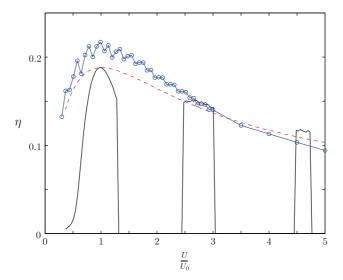
**Fig. 13.** Sensitivity of the efficiency  $\eta$  to flow speed variations for the three flexible devices considered: the tensioned cable with constant tension (solid line), the tensioned cable with a drag-induced tension (dashed line) and the hanging cable (line and symbols).
