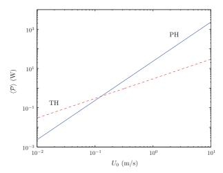
**Fig. 12.** Dimensional power,  $\langle P \rangle$  (in W), harvested by one harvester for VIV of a tensioned cable with periodically-distributed energy harvesters (solid line) or a hanging cable (dashed line). For each flow velocity  $U_0$  and each configuration, the optimal dimensional parameters are derived and give access to the optimal power  $\langle P \rangle$  which is extracted by a single harvester.
