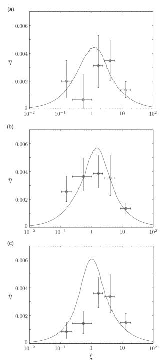
**Fig. 8.** Efficiency  $\eta$  obtained experimentally (symbols) and by the model for VIV of a hanging string (solid line) for (a)  $\ell$  = 15.0, (b)  $\ell$  = 34.1 and (c)  $\ell$  = 50.0.
