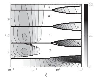
**Fig. 5.** Efficiency  $\eta$  as a function of  $\xi$  and  $\ell$ . The white cross locates the optimal harvesting configuration:  $\xi$ =3.65 and  $\ell$ =0.55, leading to an efficiency of  $\eta$ =0.19. The number of the dominant mode, determined by a linear stability analysis, is also indicated and the heavy lines mark the boundaries between the dominance zones of each mode number.
