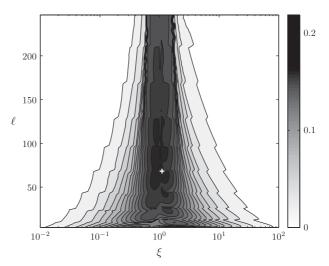
**Fig. 9.** Efficiency of the energy harvesting by VIV of a hanging cable with a single dashpot localized at its upper end as a function of the damping parameter  $\xi$  and reduced length  $\ell$ . The white cross locates the optimal harvesting configuration:  $\xi$ =1.1 and  $\ell$ =68.3, leading to an efficiency of  $\eta$ =0.22.
