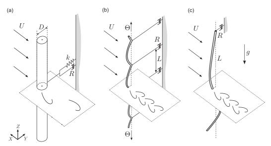
**Fig. 1.** Energy harvesting by cross-flow VIV of (a) an elastically-mounted rigid cylinder, (b) a tensioned cable with periodically-distributed energy harvesters and (c) a hanging cable with a single energy harvester at its upper extremity.
