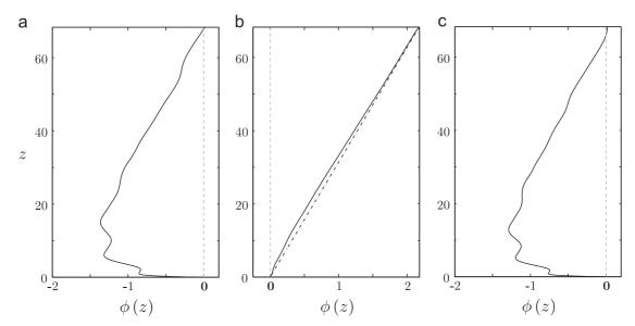
**Fig. 11.** Energy flux  $\phi(z)$  for (a)  $\xi = \xi_{opt}/100$ , (b)  $\xi = \xi_{opt}$  and (c)  $\xi = 100\xi_{opt}$ . The dashed-dotted line shows the linear approximation of  $\phi$  on plot (b).
