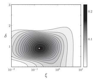
**Fig. 2.** Efficiency of the energy harvesting by VIV of an elastically-mounted rigid cylinder, as a function of the damping parameter  $\xi$  and the frequency ratio  $\delta$ . The white cross locates the optimal harvesting configuration:  $\xi$ =0.16 and  $\delta$ =0.90, leading to an efficiency of  $\eta$ =0.23.
