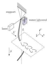
Fig. 7. Sketch of the experimental setup for the analysis of the energy harvesting by cross-flow VIV of a hanging cable in a uniform flow.
