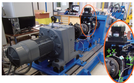
Figure 1: A picture of the wind turbine test bench. The orange ellipsis circles zooms in the main bearing and its loading unit, while the green arrows represents the 3 wired accelerometers.
