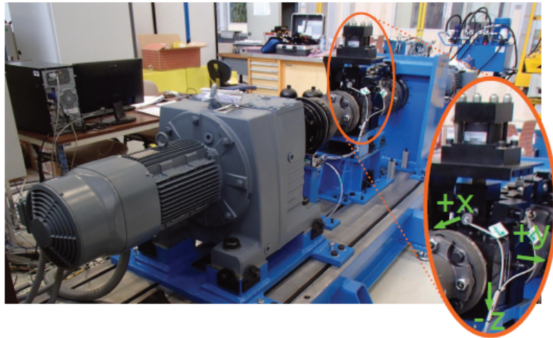
Figure 2: A picture of the test rig. The main bearing is marked by an orange ellipsis and the three accelerometer directions are symbolized by the green arrows.
