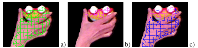
Fig. 7 Connected entities recognition: a) all extracted mid-features (HSV pairs); b) the mid-features of the first recognized view, c) the mid-features of the first recognized view (shown by pink color) and the mid-features of the connected view (shown by blue color).
