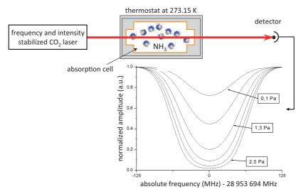
Fig. 1. The Doppler Broadening Technique principle.
