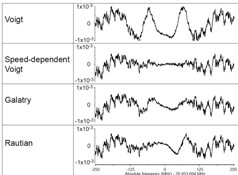
**Fig. 2.** Normalized residuals for nonlinear least-squares fits of the same average of 24 spectra, recorded at 17.3 Pa, to the exponential of a Voigt, a speed-dependent Voigt, a Galatry and a Rautian profile.
