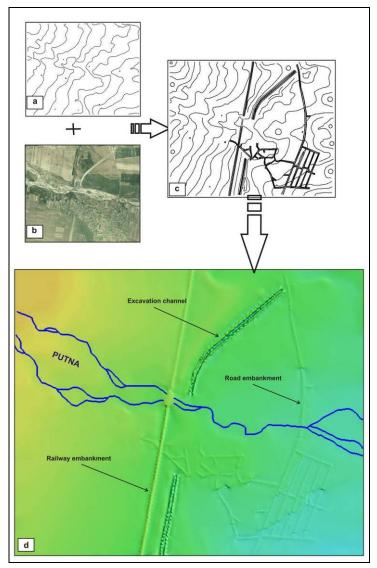
Fig. 1 a – contour lines; b – orthofotomap, year 2005; c – contour lines + isolines resulted from the updated information; d – anthropogenic landforms represented on the digital elevation model.
