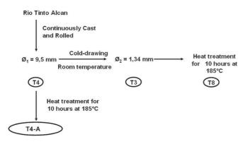
Figure 1. Forming process of the AA6101 strands.
