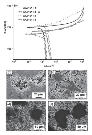
**Figure 5.** (a) Current-potential curves of the AA6101 T4, T4-A, T3 and T8 samples in a 0.5 M NaCl solution. Scan rate = 500 mV. h<sup>-1</sup>. SEM observations after polarization tests of (b) the T4 samples (c) the T4-A samples. OM observations after polarization tests of (d) the T3 samples and (e) the T8 samples.
