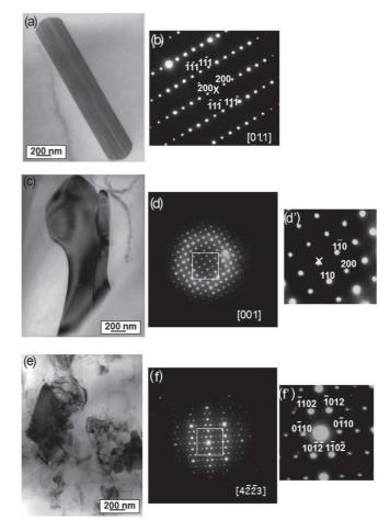
**Figure 4.** TEM observations of the microstructure of AA6101 T4 (a)  $Al_9Fe_2Si_2$  compound (b) selected area diffraction pattern analysis of  $Al_9Fe_2Si_2$  compound (c)  $Al_{17}(Fe,Mn)_4Si_2$  compound (d) and (d') selected area diffraction pattern analysis of  $Al_{17}(Fe,Mn)_4Si_2$  compound (e)  $Al_7Fe_2Si$  compound (f) and (f') selected area diffraction pattern analysis of  $Al_7Fe_2Si$  compound (f) and (f') selected area diffraction pattern analysis of  $Al_7Fe_2Si$  compound.
