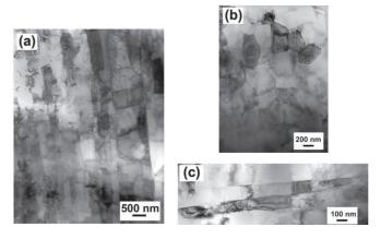
Figure 9. (a), (b) and (c) TEM observations of the AA6101 T8 samples.
