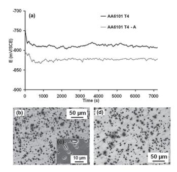
**Figure 2.** (a) OCP measurements of AA6101 T4 and T4-A in a 0.5M NaCl solution (b) OM observations of the T4 samples after OCP (c) SEM observations of the T4 samples after OCP: zoom on intermetallic particles (d) OM observations of T4-A metallurgical state after OCP.
