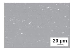
Figure 3. SEM observations of the microstructure of AA6101 T4 in transverse plane.
