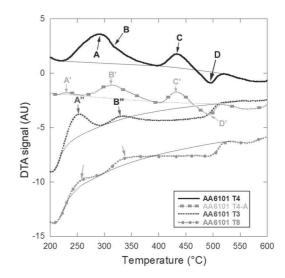
Figure 7. DTA curves for the AA6101 T4, AA6101 T4-A, AA6101 T3 and AA6101 T8 samples. The baseline is plotted for more clarity.
