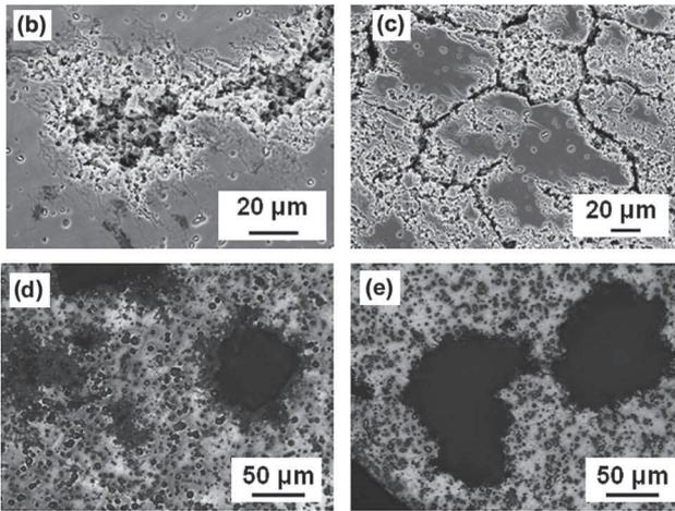
**Figure 5.** (a) Current-potential curves of the AA6101 T4, T4-A, T3 and T8 samples in a 0.5 M NaCl solution. Scan rate = 500 mV. h<sup>-1</sup>. SEM observations after polarization tests of (b) the T4 samples (c) the T4-A samples. OM observations after polarization tests of (d) the T3 samples and (e) the T8 samples.
