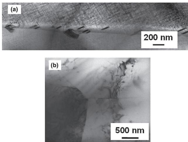
**Figure 6.** (a) TEM observation of a grain boundary of the AA6101 T4-A microstructural state (b) TEM observation of a grain boundary of the AA6101 T4 sample.
