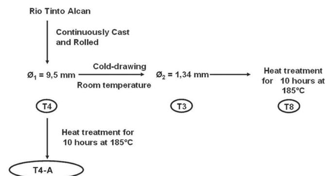
**Figure 1.** Forming process of the AA6101 strands.
