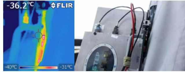
Fig. 15 Photographs of the ASTEP camera box at the interface with the telescope. Left: IR photograph showing the warm plume at the interface between the camera box and the telescope tube. Right: Visible photograph of the camera box and telescope tube.
