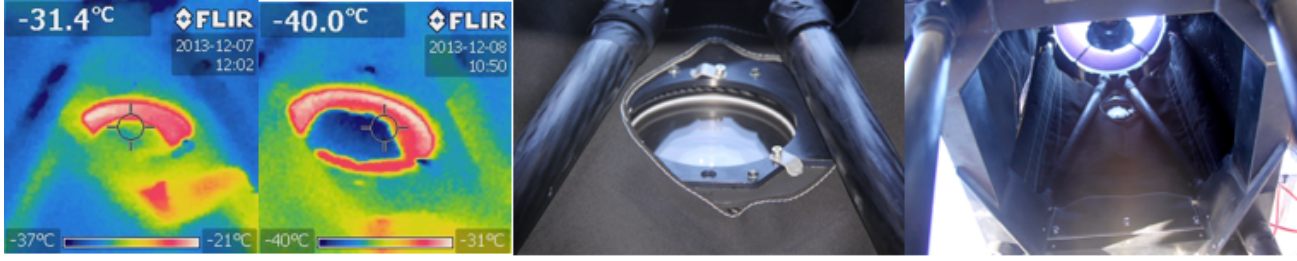
Fig. 14 Photographs of the camera entrance window in the infrared and visible. First photograph from the left: Camera box entrance window in the IR when heated to +10^{\circ}\text{C} inside the camera box. Second photograph: Camera window in the IR when heated -8^{\circ}\text{C} (2nd IR image). Third photograph: Blowup of the camera window in the visible to scale with the IR photographs. Fourth photograph: Visible photograph is taken from near the M1 mirror, looking up towards the camera window and the M2 mirror.
