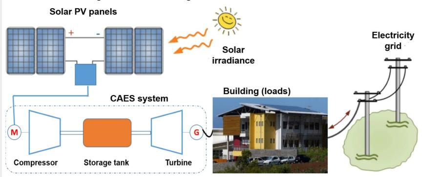
The excess electricity producted by the PV is used to power the compressor for storing compressed air in a tank. This air will be used to power an air turbine to power the building's loads when demand rises or will be injected to the electric grid, different scenarios will be studied.
