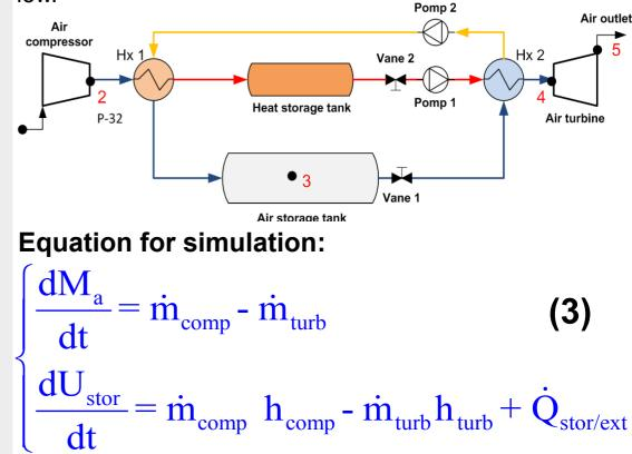
The equivalent equation is used to calculate the heat storage system, taking into account the eventual loss in the tank and at the heat exchangers. A dynamic coupling of CAES with a building and a renewable energy generation (photovoltaic) will be studied.
