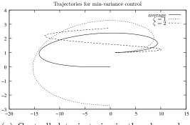
(a) Controlled trajectories in the phase plan using the optimal control for  $\kappa = 5.10^3$ . The variance at final time is 7.41.
