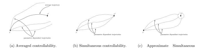
Figure 1: Different controllability notions, introduced in (1.5), (1.6) and (1.7), for parameter dependent systems, with initial condition and target independent of  $\zeta$ .
