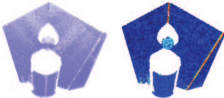
Figure 2. Example of data provided by the scanner: 2D image and 3D coordinates
