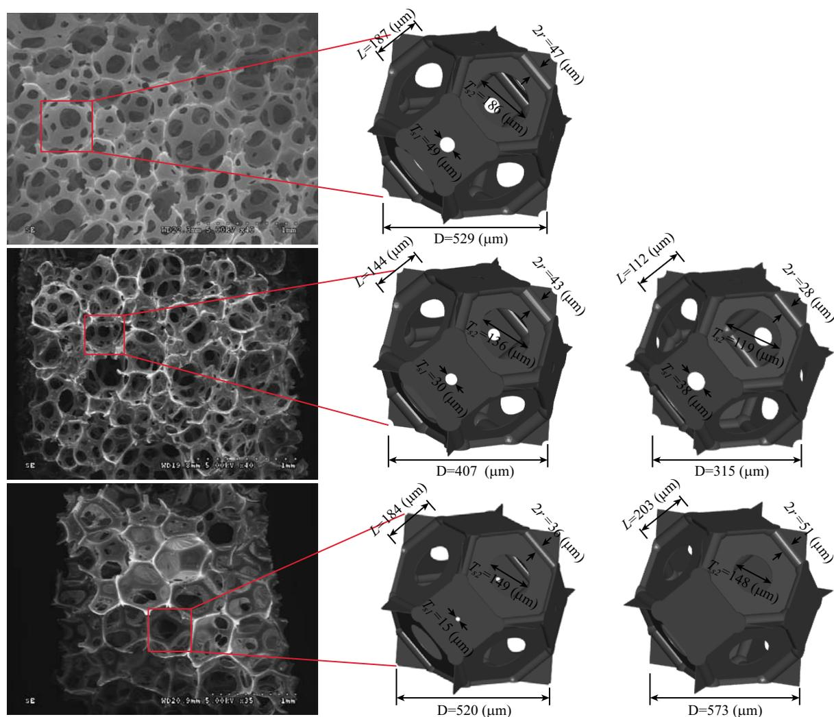
Figure 1 : Cellular structure modifications: (upper)  $H_0$  standard, (central)  $H_{1b}$  sound insulating, and (lower)  $H_{2b}$  sound absorbing foams. Scanning electron micrographs (left), identification of the local characteristic lengths corresponding to the foams as manufactured (middle), and recommended feasible cellular designs to produce the targeted sets of poroelastic parameters (right).
