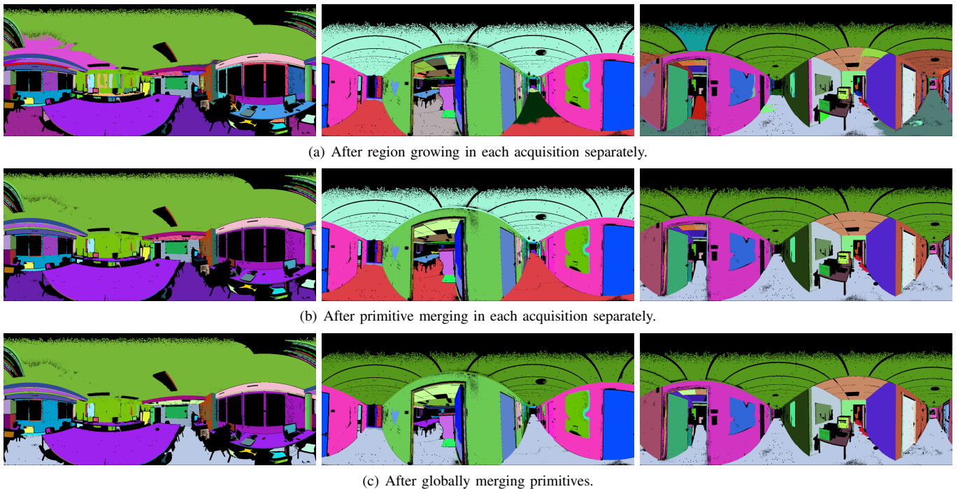
Fig. 4. Plane merging on multiple laser acquisitions (one color per segment): fusion is first applied to each acquisition separately, then globally (with \delta = 0.01 ).
