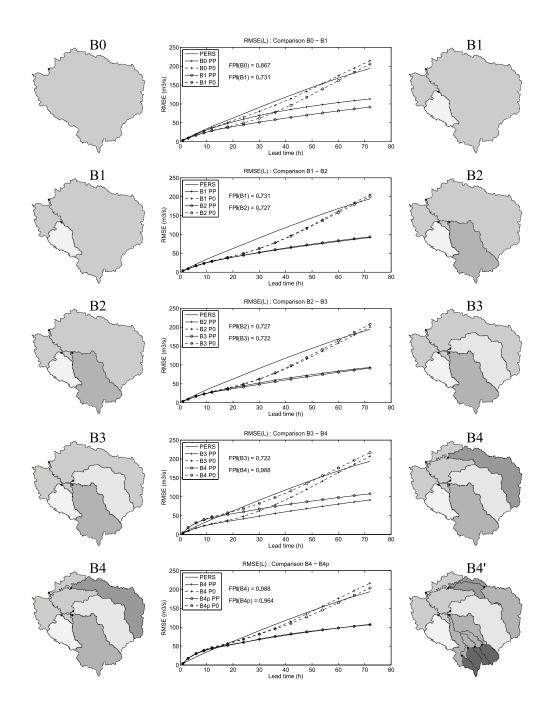
FIG. 12. Forecast performance obtained in validation by the TGR model and the persistence model (PERS) at the Paris-Austerlitz station for the B configurations using PP and P0 rainfall scenarios. Lead times range from 1 to 72 hours. Two configurations are compared in each case, illustrated on the left and right hand sides of the graph.
