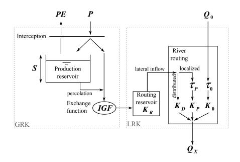
FIG. 6. The TGR coupled model scheme for one intermediate basin.
