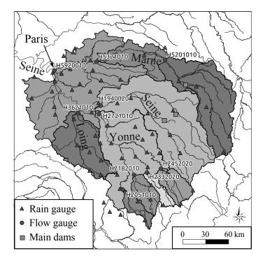
FIG. 1. The Seine River basin at Paris (43,800  $\text{km}^2$ ), and the networks of raingauges and flow gauging stations used in the study. The station details corresponding to the codes shown on the map are given in Table 1.
