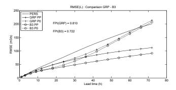
FIG. 15. Forecast performance obtained in validation by the TGR model (configuration B3), the GRP model and the persistence model (PERS) at the Paris-Austerlitz station using PP and P0 rainfall scenarios. Lead times range from 1 to 72 hours.
