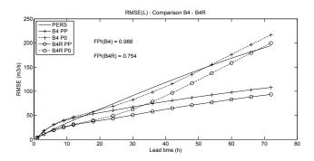
FIG. 13. Forecast performance obtained in validation by the TGR model with configurations B4 and B4R, and the persistence model (PERS) at the Paris-Austerlitz station using PP and P0 rainfall scenarios. Lead times range from 1 to 72 hours.
