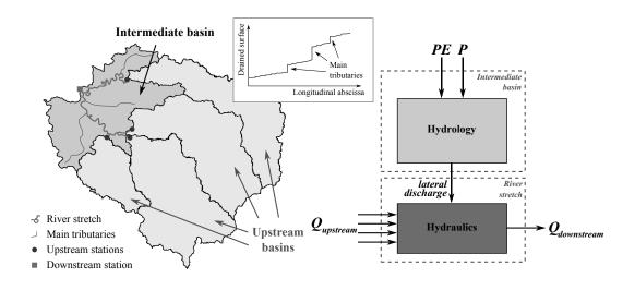
FIG. 2. Schematic representation of the hydrology-routing coupled model (PE and P are the potential evapotranspiration and rainfall inputs to the model, Q stands for streamflow). The drained area curve is used for the spatial discretization inside the intermediate basin.
