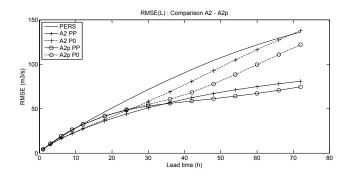
FIG. 9. Forecast performance obtained in validation by the TGR model and the persistence model (PERS) at the Courlon-sur-Yonne station for the A2 and A2' configurations using PP and P0 rainfall scenarios. Lead times range from 1 to 72 hours.
