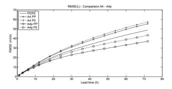
FIG. 10. Forecast performance obtained in validation by the TGR model and the persistence model (PERS) at the La Ferté-sous-Jouarre station for the A4 and A4' configurations using PP and P0 rainfall scenarios. Lead times range from 1 to 72 hours.
