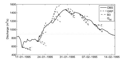
FIG. 16. Example of discharge forecast by the TGR model (configuration B3) and the GRP operational model during the 1995 main flood event with a 72-hour lead time and for PP and P0 scenarios.
