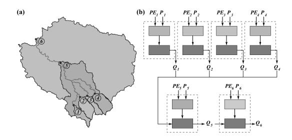
FIG. 3. (a) Example of hydrological discretization based on the gauging station network and (b) corresponding modelling scheme.
