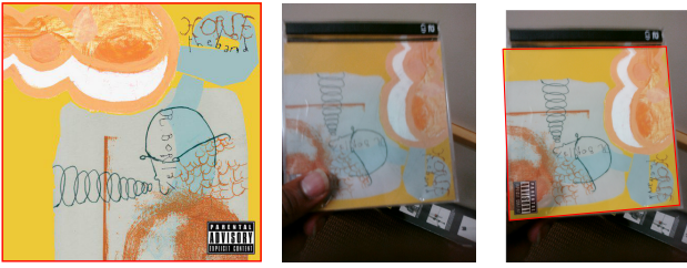
Fig. 13. Homographic registration of a pair of images. Left: reference image. Middle: target image. Right: registration result using TBMR. None other tested detector yields a correct registration.
