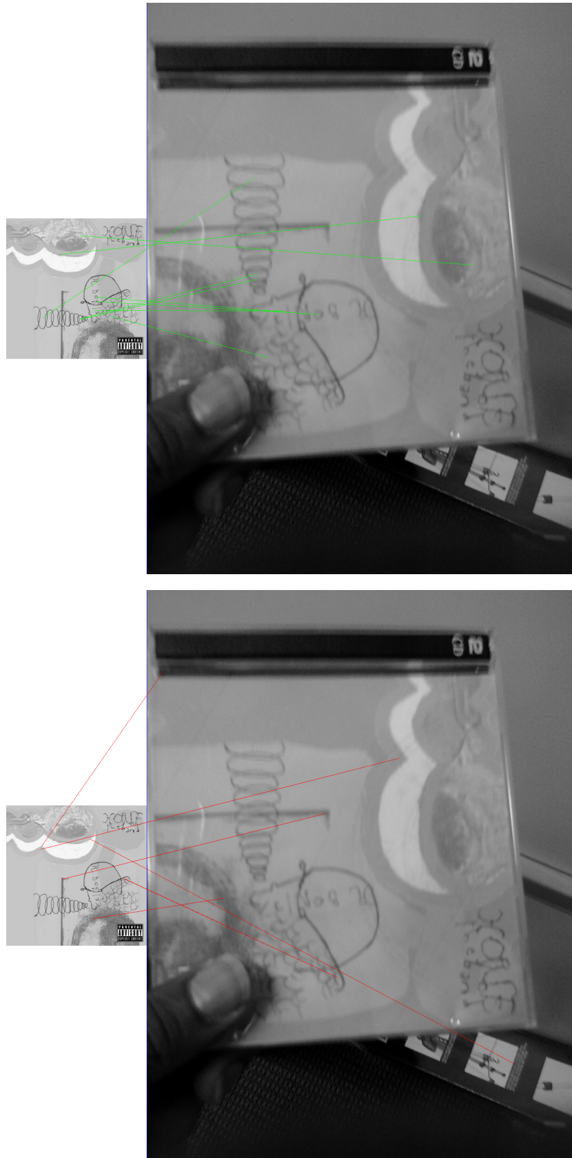
Fig. 8. Matched pairs of points using respectively TBMR (top) and DoG (down). All the matched pairs of points using TBMR are used as inliers to estimate the homography. Using DoG fails to estimate the homography: all the matched pairs of points are considered as outliers. Though four pairs are correct, there is no other to check automatically the resulting homography.
