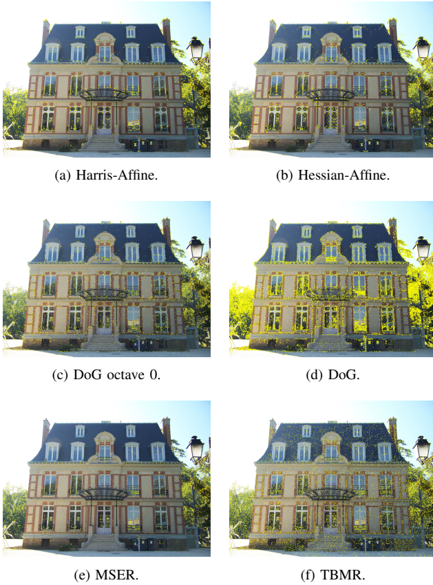
Fig. 4. Qualitative comparison of TBMR with other widely used local feature detectors applied on an image taken against the sunlight (used in Figure 1). Yellow points in the image are the detected keypoints.
