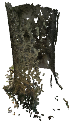
(b) 3D result using DoG, 13 images are calibrated.
