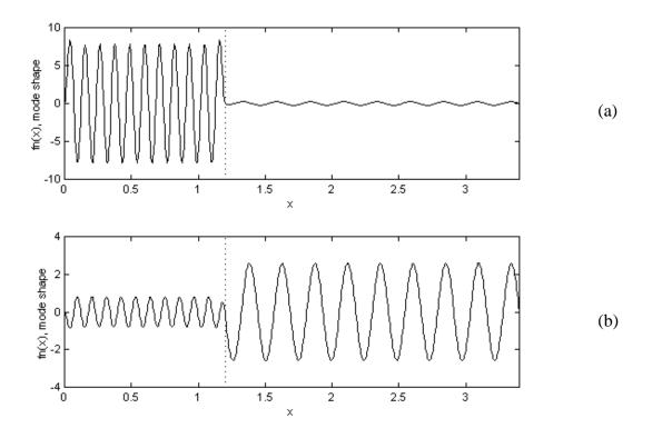
Figure 13. Examples of displacement mode shapes for subsystem 2. (a) mode 1 of the previous figure; (b) mode 2 of the previous figure.
