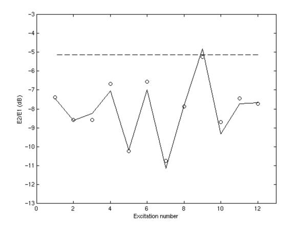
Figure 15. Total energy ratio for each excitation point. Third octave band of central frequency 1000 hz. Comparison of three calculations : o, reference obtained from DMF with non resonant modes ; \_\_\_\_\_, SmEdA ; ----, SEA.
