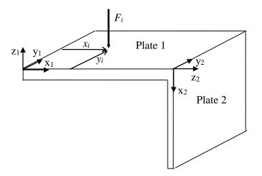
Figure 14. Two plates coupled in an L-shape and excited by a point force  $F_i$  on plate 1.  $a_1=1,7$  m,  $a_2=0,8$  m, b=1 m,  $h_1=6$  mm,  $h_2=3$  mm,  $E_1=E_2=2.10^{11}$  Pa,  $\rho_1=\rho_2=7800$  kg/m<sup>3</sup>,  $\eta_1=\eta_2=0,01$ .
