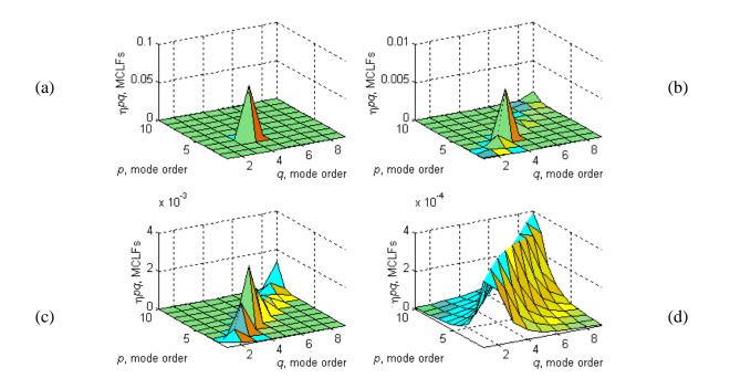
Figure 7. Modal coupling loss factors,  $\eta_{pq}$ . (Modes classified with increasing natural frequencies.) Same cases than the previous figure : (a)  $\overline{M} = 7,9.10^{-3}$ ; (b)  $\overline{M} = 0.09$ ; (c)  $\overline{M} = 0.18$ ; (d)  $\overline{M} = 1.43$ .
