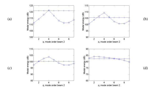
Figure 6. Modal energy distribution of the receiving beam (dB, ref.  $10^{-12}$  joule). Resonant modes classified with increasing natural frequencies. Four cases : (a)  $\overline{M} = 7,9.10^{-3}$ ; (b)  $\overline{M} = 0.09$ ; (c)  $\overline{M} = 0.18$ ; (d)  $\overline{M} = 1.43$ . Two calculations : -o-o-, SmEdA ; -+-+-, SEA<sup>DMF</sup>.
