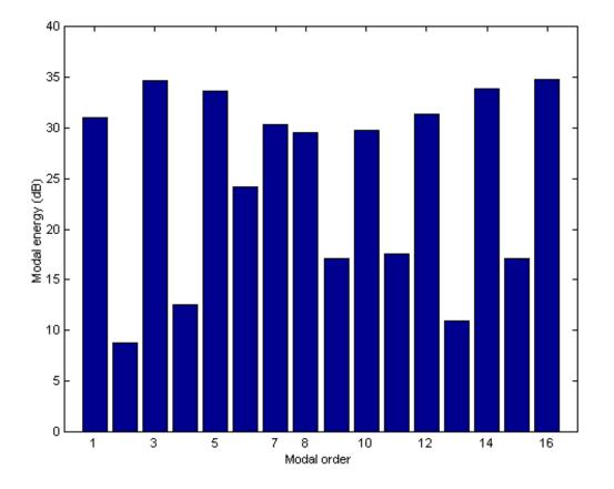
Figure 12. Modal energy distribution of subsystem 2 (dB, ref.  $10^{-12}$  joule). Modes classified with increasing natural frequencies. SmEdA results.
