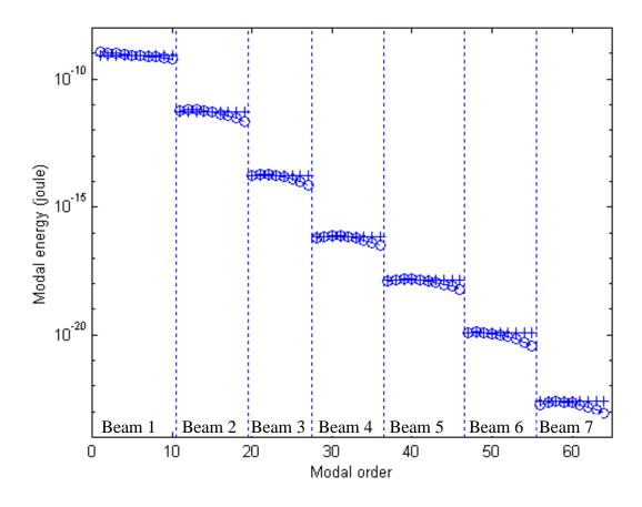
Figure 10. Modal energy distributions of the 7 beams in the case of geometric mean modal overlap factors equal to one:  $\eta_{\alpha}=0.08$ ,  $\alpha \in [1,7]$ . Octave band of central frequency 1000 Hz. Two calculations : -o-o-, SmEdA ; -+-+-, SEA<sup>DMF</sup>.
