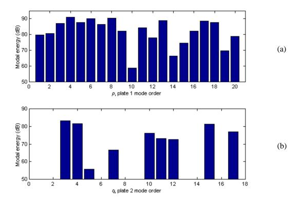
Figure 16. Modal energy distributions for excitation case number 7 (dB, ref.  $10^{-12}$  joule). (a) Plate 1. (b) Plate 2. Modes classified with increasing natural frequencies.
