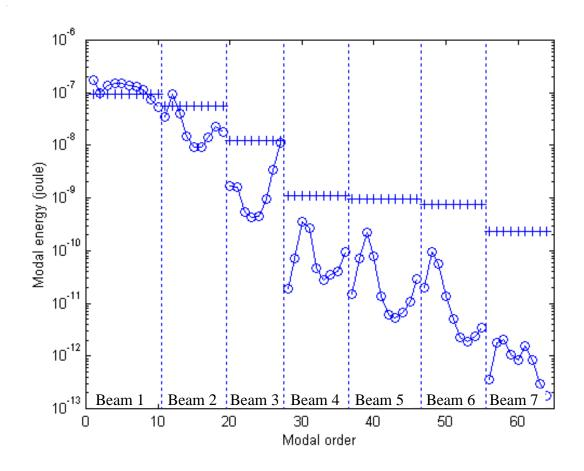
Figure 9. Modal energy distributions of the 7 beams in the case of weak modal overlap:  $\eta_{\alpha}$ =0.001,  $\alpha \in [1,7]$ . Octave band of central frequency 1000 Hz. Two calculations: -o-o-, SmEdA; -+-+-, SEA<sup>DMF</sup>.
