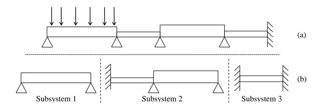
Figure 11. (a) Illustration of the 4 coupled beams; (b) Substructuring. Beams' characteristics: L<sub>1</sub>=2,4 m, L<sub>2</sub>=1,2 m, L<sub>3</sub>=2,2 m,L<sub>4</sub>= 1,4m, h<sub>1</sub>=3 mm, h<sub>2</sub>=1 mm, h<sub>3</sub>=5 mm, h<sub>4</sub>=1,2 mm, b<sub> $\alpha$ </sub>= 0,01 m, E<sub> $\alpha$ </sub> =7.10<sup>10</sup> Pa,  $\rho_{\alpha}$ =2700 kg/m<sup>3</sup>,  $\eta_{\alpha}$ =0.01 ( $\alpha \in [1,4]$ ).
