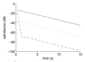
FIG. 3: Impulse responses of a  $D_4^{\#}$  string connected to the bridge and the soundboard. Solid:  $Y_{yy}^s(t)$  or  $Y_{zz}^s(t)$  (string alone direct response); dashed:  $Y_{zz}(t)$  (compound system direct response) ; dotted:  $Y_{zy}(t)$  (compound system cross response).
