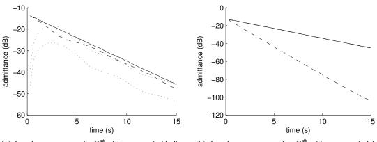
(a) Impulse responses of a  $D_4^{\#}$  string connected to the bridge. Solid:  $Y_{yy}^s(t)$  or  $Y_{zz}^s(t)$  (string alone); dashed:  $Y_{yy}(t)$  or  $Y_{zz}(t)$ ; dotted:  $Y_{zy}(t)$  (high) and  $Y_{yz}(t)$  (low)
