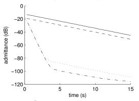
FIG. 4: Impulse responses of two  $D_4^{\#}$  strings connected to the soundboard for two different relative mistuning amounts. Solid:  $Y_{yy}^s(t)$  or  $Y_{zz}^s(t)$  (single string direct response); dashed:  $Y_{yy}(t)$ : compound system direct response in *y*-direction; dashed-dotted:  $Y_{zz}(t)$ : direct response in the *z*-direction for a 2-cents mistuning; dotted:  $Y_{zz}(t)$ : direct response in the *z*-direction for a 4-cents mistuning.
