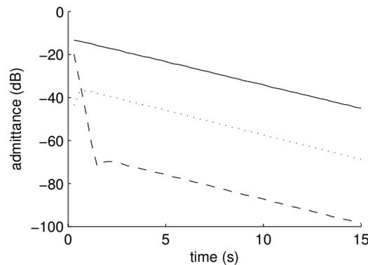
FIG. 3: Impulse responses of a  $D_4^\#$  string connected to the bridge and the soundboard. Solid:  $Y_{yy}^s(t)$  or  $Y_{zz}^s(t)$  (string alone direct response); dashed:  $Y_{zz}(t)$  (compound system direct response); dotted:  $Y_{zy}(t)$  (compound system cross response).
