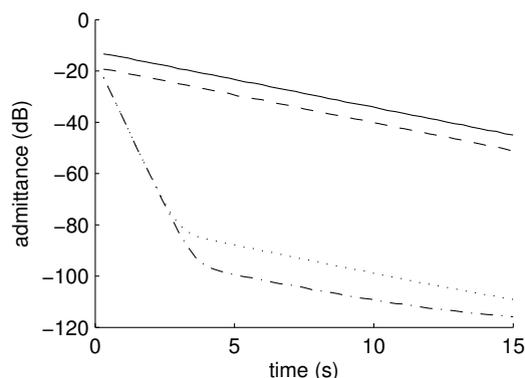
FIG. 4: Impulse responses of two  $D_4^\#$  strings connected to the soundboard for two different relative mistuning amounts. Solid:  $Y_{yy}^s(t)$  or  $Y_{zz}^s(t)$  (single string direct response); dashed:  $Y_{yy}(t)$ : compound system direct response in  $y$ -direction; dashed-dotted:  $Y_{zz}(t)$ : direct response in the  $z$ -direction for a 2-cents mistuning; dotted:  $Y_{zz}(t)$ : direct response in the  $z$ -direction for a 4-cents mistuning.
