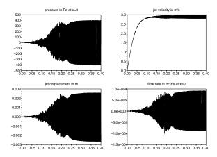
Fig. 2. Simulation results with  $p_f = 5 Pa$  and L = 0.20 m
