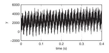
Fig. 4. Simulation of the system (-) and the observer (--) from the measured output y (-). The simulations are performed for the following parameters:  $a=150s^{-1}$ ,  $\chi=160s^{-1}$ , L=1,  $p_m=1.5e4Pa$ ,  $\omega=535s^{-1}$ , quasi-ideal initial conditions  $\hat{x}(0)=[1e-3,1e-1,\frac{y(0)}{1+\lambda}]^T$  and large noise  $\sigma_{noise}/p_m=4e-2$ .
