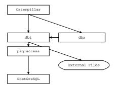
Figure 4. Architecture of the database interface.
