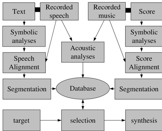
**Figure 1.** Architecture of the hybrid concatenative synthesis system.
