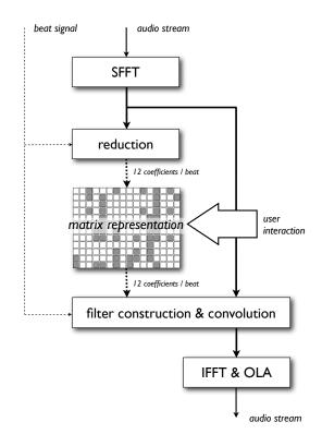
Figure 4: Data-flow diagram of the beat-synchronous processing of the X-Micks application.
