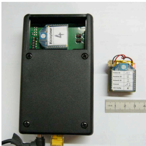
Figure 1. Right: the module with Xbee, battery and sensors (on the back of the module). Left: receptor, showing the Ethernet and power supply connectors.
