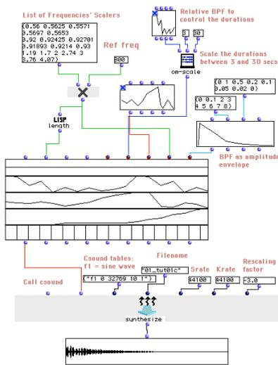
**Figure 3.** Csound additive synthesis in OMChroma. The matrix can be instantiated in different ways (functions, bpf, numerical values, lists), and then is formatted for the synthesizer by the *synthesize* generic function.
