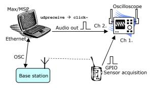
Figure 3. Latency measurement technique
