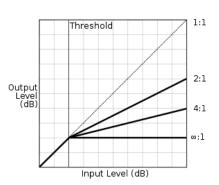
Figure 1: Relationship between input and output level in a compressor for a fixed threshold and various ratios.
