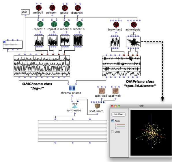
Figure 4: A spatial sound synthesis process carried out by merging the OMChroma class *fog-1* (for granular synthesis) with the OMPrisma class *spat.3d.discrete* for ambisonic spatialization. Both sound synthesis and spatialization parameters are controlled via stochastic processes.
