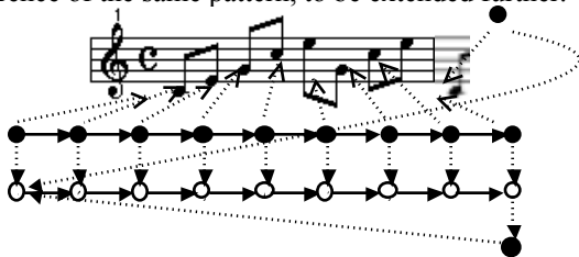
Fig. 6. When a pattern is repeated more than twice, the last note of the pattern is linked to the first note through an additional POC on the PCC.
