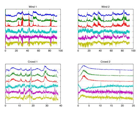
Fig. 5. Normalised descriptors for each sound file over time [s]. From top to bottom: Loudness, Harmonic Energy, Noise Energy, Spectral Spread, Perceptual Spectral Slope, Spectral Centroid.
