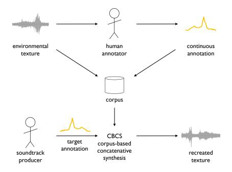
Fig. 1. Overview schema of the basic retexturing workflow.
