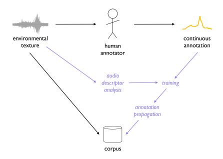
Fig. 2. Overview schema of annotation propagation workflow (light grey/blue parts in italics).
