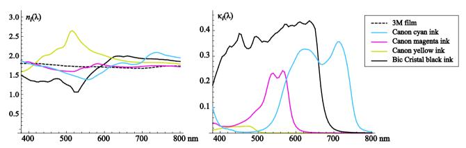
Fig. 7. Real part (left) and imaginary part (right) of the refractive index of inks as a function of wavelength.
