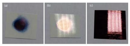
Fig. 2. Two samples of black ballpoint pen ink coated on the a glossy paper: (a-b) a thick layer at the center of the paper, surrounded by a thinner layer, is observed out of (a) and in (b) the specular direction in respect to the lamp; (c) coppered metallic reflection on a thick ink layer covering the paper.
