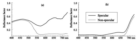
Fig. 4. Spectral reflectance factors of (a) cyan inkjet ink and (b) black ballpoint pen ink on glossy white paper, measured in steps of 10 nm in a 45°:45° geometry (black lines) or a 35°:45° geometry grey lines.
