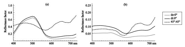
Fig. 5. Spectral reflectance factors of cyan ink coated on (a) glossy white paper and (b) a transparency film, measured in steps of 10 nm in either a de:8° geometry, a di:8° geometry, or a 45°:45° geometry.
