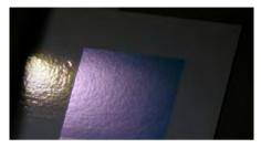
Fig. 1. Picture of a patch of cyan inkjet ink printed on a glossy paper with specular reflection of the white source. On the inked area, the specularly reflected light exhibits a pinkish sheen.
