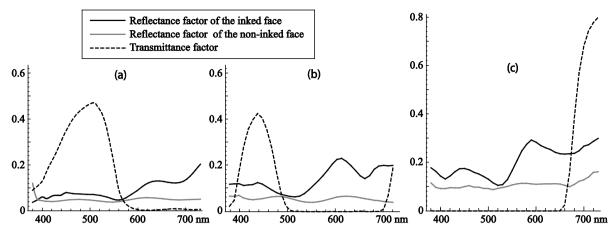
Fig. 3. Spectral reflectance and transmittance factors of a clear film coated with (a) cyan inkjet ink, (b) blue ballpoint pen ink, and (c) black ballpoint pen ink. The spectral reflectance factors are measured in the 45°:45° geometry on the inked and non-inked faces of the film. The spectral transmittances are measured in the normal direction of the film.
