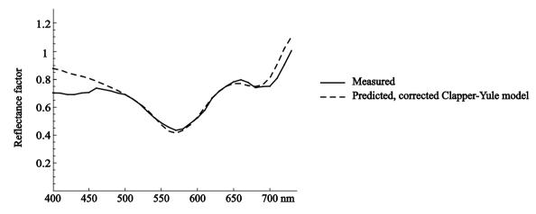
Fig. 9. The spectral reflectance factors of a photo paper coated with cyan ink measured in 45°:45° geometry is compared to the predicted spectral reflectance of the air-ink interface, computed from the complex refractive index of the ink.
