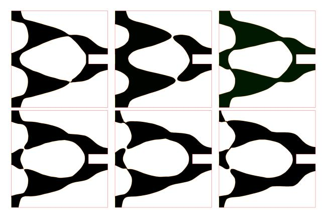
FIGURE 19. Optimal shapes in the test case of section of Section 5.2.4, associated to values of  $\beta$  (from left to right, top to bottom) 0, 0.5, 1, 1.5, 2, 2.5.
