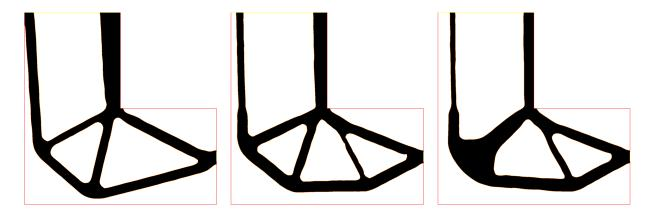
FIGURE 22. Section 5.2.5: optimal shapes in the minimization of the objective function (5.8), where the parameter  $\delta$  equals (from the left to the right) 0,0.5,2.
