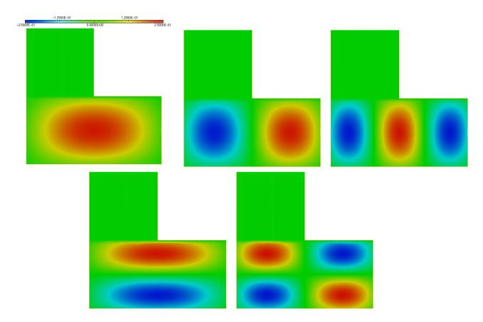
FIGURE 21. Section 5.2.5: plots of the first five eigenfunctions  $v_i$  of the correlation (5.7), retained in the approximation of the random perturbation field  $v(x, \omega)$ . The common scale to the five plots is displayed on the first one.
