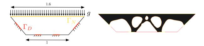
FIGURE 16. Section 5.2.3, bridge with an uncertain frequency load: (left) details of the test-case, (right) initial shape.
