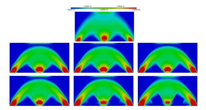
FIGURE 6. Test-case of Section 5.1.3: minimization of the failure probability (3.23); from left to right, top to bottom, unperturbed design, and optimal thicknesses associated to the values  $\alpha = 0.0017, 0.0018, 0.0019, 0.002, 0.0025, 0.003$ .
