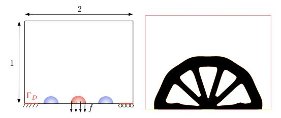
FIGURE 8. Section 5.2.2: (left) description of the bridge test case, (right) optimal shape in the unperturbed situation.
