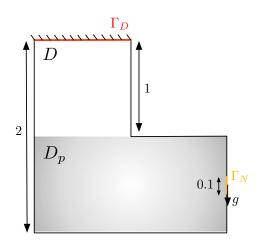
FIGURE 20. Section 5.2.5: details of the L-shaped beam test-case.
