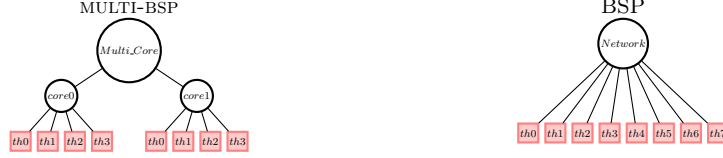
Fig. 4 The difference between the MULTI-BSP and BSP models for a multicore architecture. (node) contains memory. Fig. 4 illustrates the difference between both models for multicores. There exist other hierarchical models [38], such as D-BSP [1] or H-BSP [7], but MULTI-BSP describes them in a simpler way. An instance of MULTI-BSP is defined by \mathbf{d} the depth of a tree and 4 parameters for each stage i :
