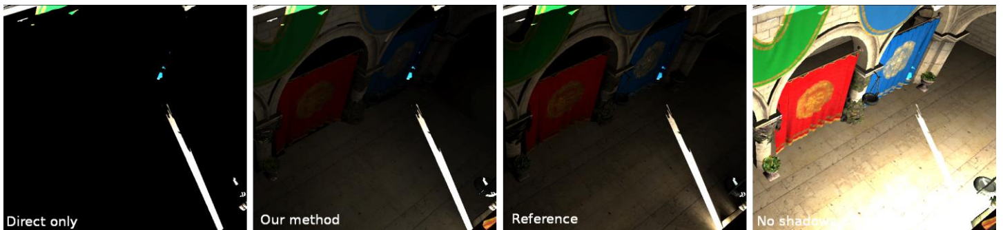
Figure 12. We compare the result of our method with a rendering that ignore shadows for the virtual point lights. When illumination is mostly indirect, like in this case, doing such an approximation can drastically affects the final image. Our method gives a result close to the reference by using a subset of VPLs well-chosen to illuminate each view sample.
