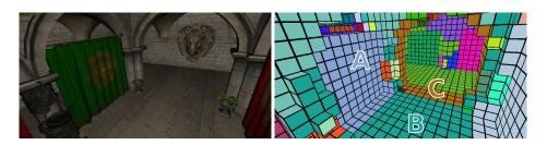
**Fig. 3.** The opening labeling of a scene. Region A is a false positive because going from B to A does not grant access to other regions of the scene and leads directly on a wall. Region C is interesting because it represents a passage to enter a corridor. It represents a hole in the 3D scene.
