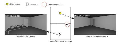
**Fig. 1.** The Ajar Door scene. The center image is a cut along the vertical axis of a voxelization of the scene. White pixels represent the empty space and black pixels represent the scene. The red circle encloses the small passage that rays must take to go from one room to the other.
