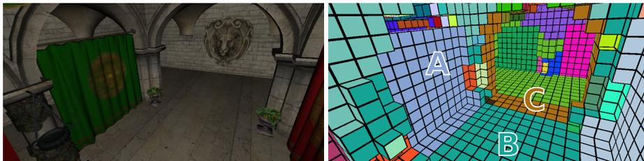
**Fig. 3.** The opening labeling of a scene. Region  $A$  is a false positive because going from  $B$  to  $A$  does not grant access to other regions of the scene and leads directly on a wall. Region  $C$  is interesting because it represents a passage to enter a corridor. It represents a hole in the 3D scene.
