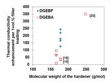
**Figure 9.** Thermal conductivity enhancement per 1% vol. filler loading versus hardener molecular mass. The hatched square is relative to our data.
