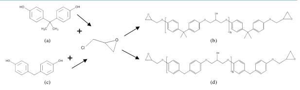
Figure 2. Chemical structures of the oligomers and resins. (a) BPA, (b) DGEBA, (c) BPF and (d) DGEBF ("n" denotes the number of polymerized subunits).
