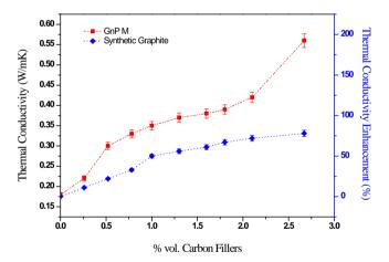
**Figure 6.** Thermal conductivity and enhancement of epoxy-DGEBA based composites at room temperature carried on synthetic graphite and GnP M fillers.
