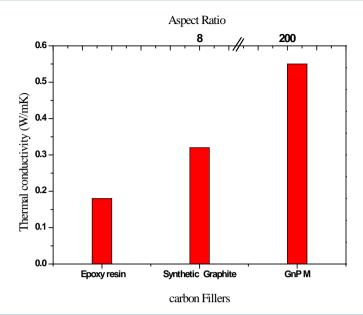
**Figure 5.** Thermal conductivities of epoxy composites at room temperature prepared with 2.67 vol % loading of graphitic fillers: GnP M, average particle size L  $\sim$  10 microns, t  $\sim$  45 nm. The thermal conductivity of pristine epoxy is included for comparison. Top scale shows the average aspect ratios of the graphite micro and nanofiller particles.
