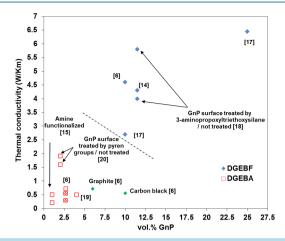
Figure 7. (a) evolution of the thermal conductivity of different epoxide system in function of the maximum volume loading fraction for each epoxy-system and process studied; (b) Influence of the Eqv./kg in the thermal conductivity (Carbon black and micronic graphite were reported as a filled losange [6] and our data as dashed squares (GnP M and Graphite: up and down respectively).
