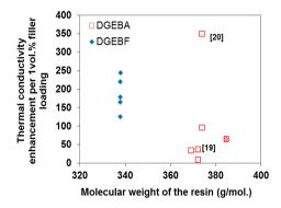
**Figure 8.** Thermal enhancement per % vol. filler loading in function of the molar mass of the epoxy resin carried out. The hatched square is relative to our data.
