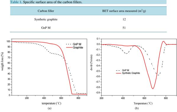
Figure 4. (a) TGA and (b) DTG curves of carbon fillers.
