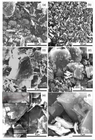
**Figure 3.** SEM images of raw powders of GnP M (a) and graphite (b) revealing overlapping regions, and grain size dispersion. Images (c) and (d) were obtained after deagglomeration by ultrasonification and deposition on silicon wafer. Images (e) and (f) were obtained at high magnification revealing overlapping and wrinkled regions. The zoom is an elementary particle folded which appears transparent at 1 kV.
