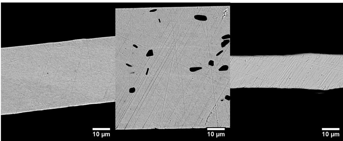
Figure 3 : BSE micrographs collected from a) the pure Cu end, b) diffusion zone and c) Co rich end of a solution treated and quenched diffusion couple. A number of dark spots ( $< 1 \mu\text{m}$ ) are visible at the Co rich end of the sample (c), and are thought to be small voids. Spot analyses of the large ( $\sim 5 \mu\text{m}$ ) inclusions found in the diffusion zone (b) indicate that they are Co oxides.
