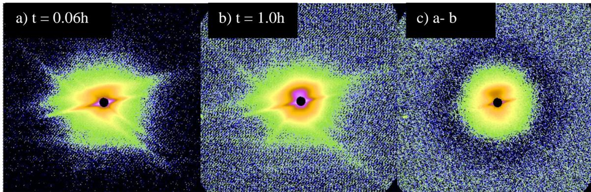
*Figure 6 : SAXS image collected from the middle of the diffusion zone of the 550°C sample. a) initial image ( $t=0.06h$ ) and b) image collected after 1h of ageing. Note the multiple intense streaks passing through or near the beamstop. c) Image after 1h minus initial image. While some streak features still appear, the signal is now mostly isotropic, as expected from spherical precipitates. The same colour scale is used for all the images.*
