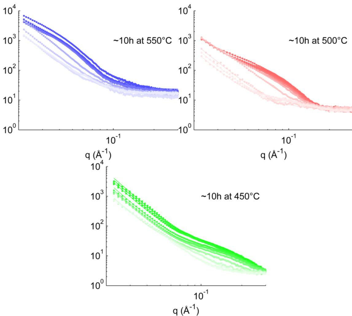
*Figure 7 : experimental SAXS patterns obtained after 10h at a) 550°C, b) 500°C and c) 450°C. The color shade is related to the local Co content (darker = more Co). The lines are the best fits according to Eq. (4).*
