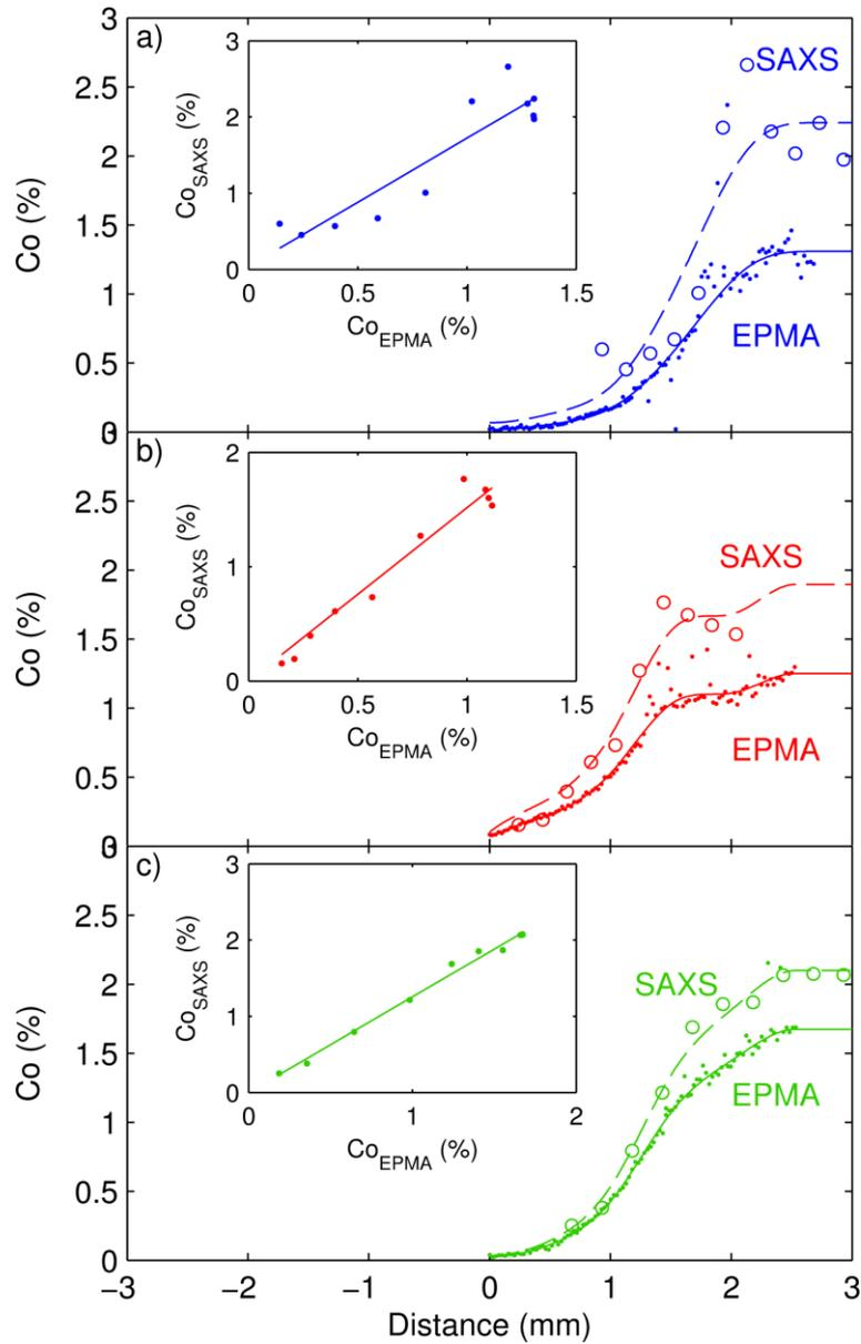
**Figure 5 : Comparison of the Co concentration profiles measured using EPMA and SAXS for the samples aged in situ at a) 550°C, b) 500°C and c) 450°C. The insets show the linear relationship between EPMA and SAXS results. The dashed trend line used for SAXS is the linearly transformed EPMA trend line.**
