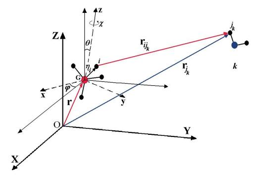
Figure 2: Geometrical characteristics of a guest molecule (CH<sub>4</sub> for instance) interacting with a water molecule of the clathrate matrix.  $(O, \mathbf{X}, \mathbf{Y}, \mathbf{Z})$  and  $(G, \mathbf{x}, \mathbf{y}, \mathbf{z})$  represent the absolute frame tied to the clathrate matrix and the molecular frame, respectively.
