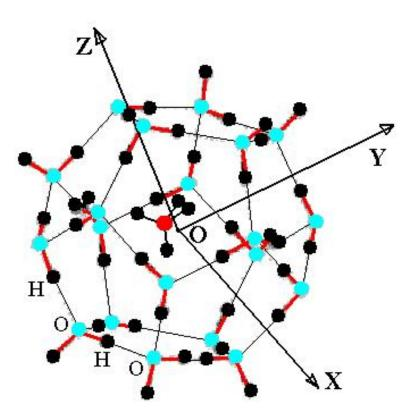
Figure 1: Trapping geometry of a guest molecule (CH<sub>4</sub> for instance) in a small cage of the structure type I.  $(O, \mathbf{X}, \mathbf{Y}, \mathbf{Z})$  represents the absolute frame tied to the clathrate lattice.
