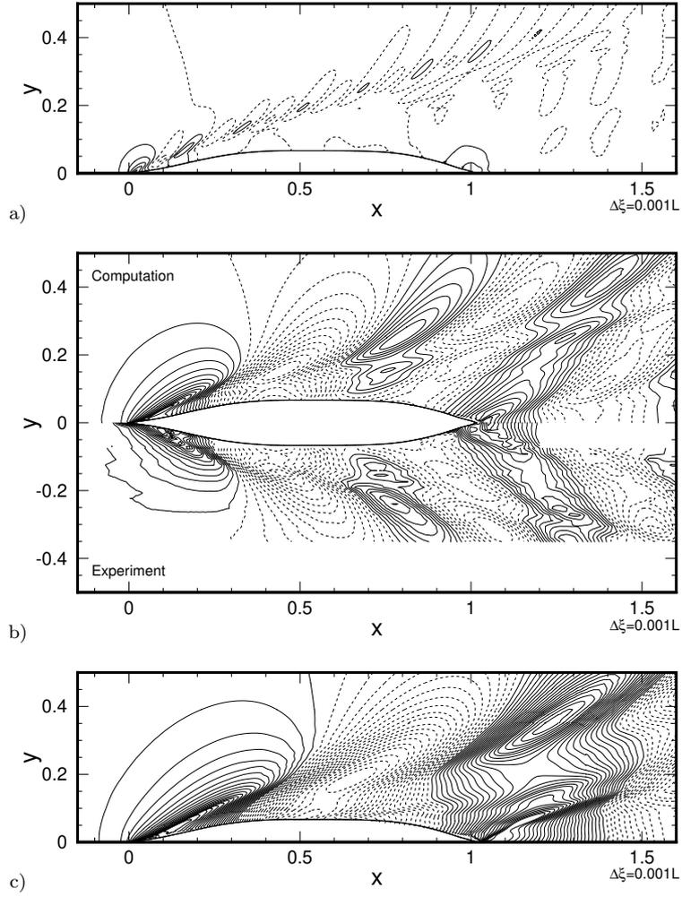
Figure 9: Wave patterns for the Series 60 at  $Fr = 0.16$  (a),  $Fr = 0.316$  (b), and  $Fr = 0.41$  (c). The isoline distance is the same for all figures and corresponds to  $L/1000$ . The  $Fr = 0.316$  result is compared with experiments from IIHR [13].
