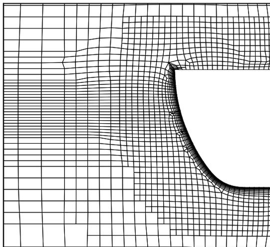
Figure 3: Cut through an unstructured hexahedral mesh.
