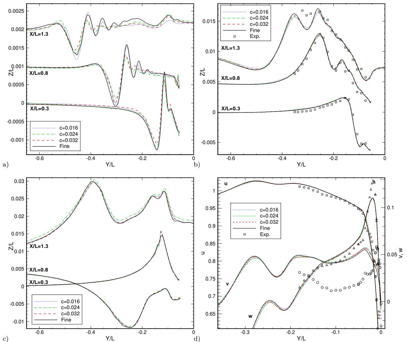
Figure 12: Series 60, comparisons of the water surface in three  $X$ -cuts at  $Fr = 0.16$  (a),  $Fr = 0.316$  (b), and  $Fr = 0.41$  (c). Comparison of the velocities on the line  $X/L = 1$ ,  $Z/L = -0.02$  (d) for  $Fr = 0.316$ . Experiments from IIHR [13].
