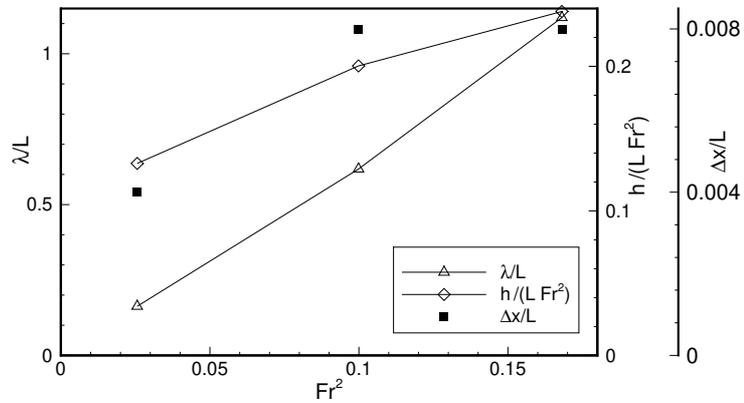
Figure 10: Nondimensional stern wave length, bow wave height, and horizontal cell size at the stern wave in the automatically refined meshes ( $c = 0.032$ ) for the Series 60 test case at different  $Fr$ .
