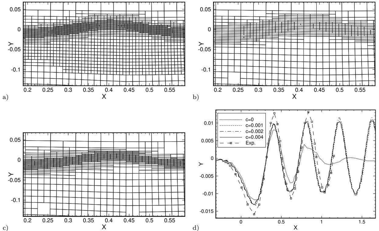
Figure 8: Refined meshes at the first wave crest for the Duncan case with  $T_r = 0.0025$ ,  $c = 0.002$  (a), with  $T_r = 0.005$ ,  $c = 0.002$  (b), and with  $T_r = 0.0025$ ,  $c = 0.001$  (c). Figure (d) compares the wave elevation for  $T_r = 0.0025$  and four different  $c$  with Duncan’s experiment [5].
