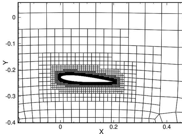
Figure 7: Original mesh for the Duncan case.
