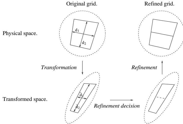
Figure 4: Tensor refinement criterion. Cell  $\Omega$  and unit circle (reference) in the physical space, deformed cell  $\tilde{\Omega}$  and deformed circle after application of the transformation  $C$ , refinement decisions to create a uniform grid in the deformed space, and the resulting anisotropically refined grid.
