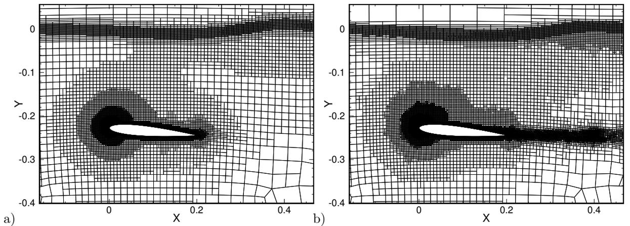
Figure 6: Refined mesh around the immersed profile for the Duncan case with  $c = 0.002$ . The Hessian is evaluated with SG (a) and LS3 (b).
