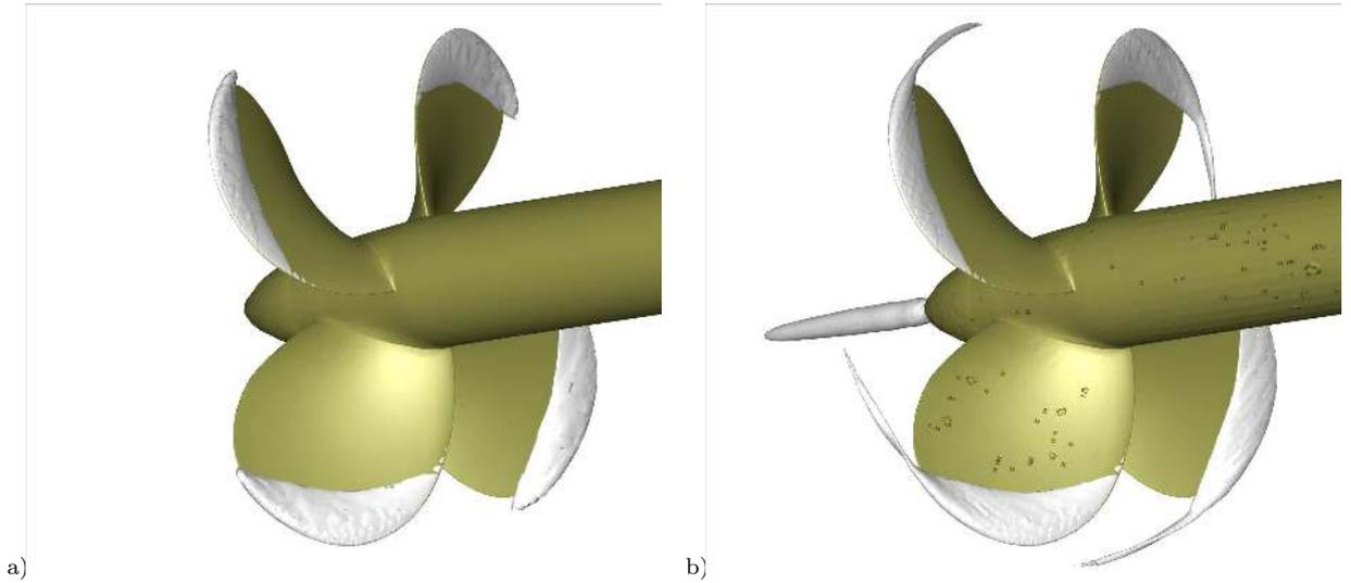
Figure 13: Computed surface of the cavitating pockets (isovalue  $\alpha = 0.5$ ) for the INSEAN E779A propeller, on the original grid (a) and the adaptively refined grid with  $T_r = 0.0012$  (b). (The small spots on the surface are plotting artefacts.)
