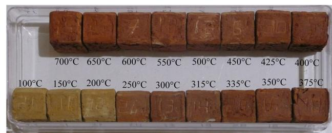
**Fig. 11** Samples of sediments from the cave of Les Fraux heated in an electric oven for 1 h at each temperature from 100 to 700 °C. The main colour modification appears at 250 °C
