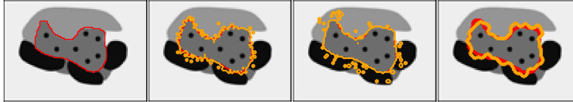
Fig. 1: From left to right: synthetic image with region of interest outlined in red; segmentation sampling based on log-odds; segmentation sampling based on STAPLE without ICM steps ( p = 68\% and q = 66\% ); ISS based on STAPLE with ICM steps ( p = 68\% and q = 66\% ). The ground truth is outlined in red, the samples are outlined in orange.
