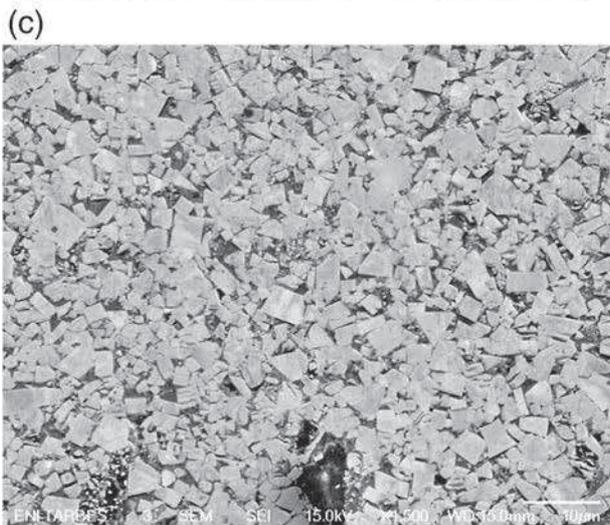
**Fig. 12.** SEM observations of the inserts worn surfaces after experiments at constant loads of 14 N (images size of 80 μm × 64 μm): a – P8; b – P12; c – P16.
