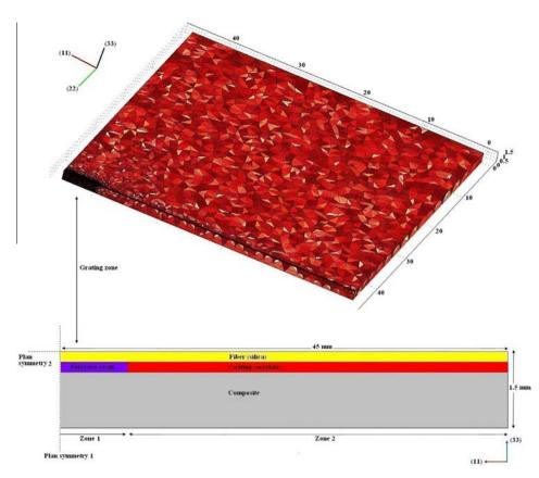
Fig. 3. Schematic view of the internal section of instrumented specimen.
