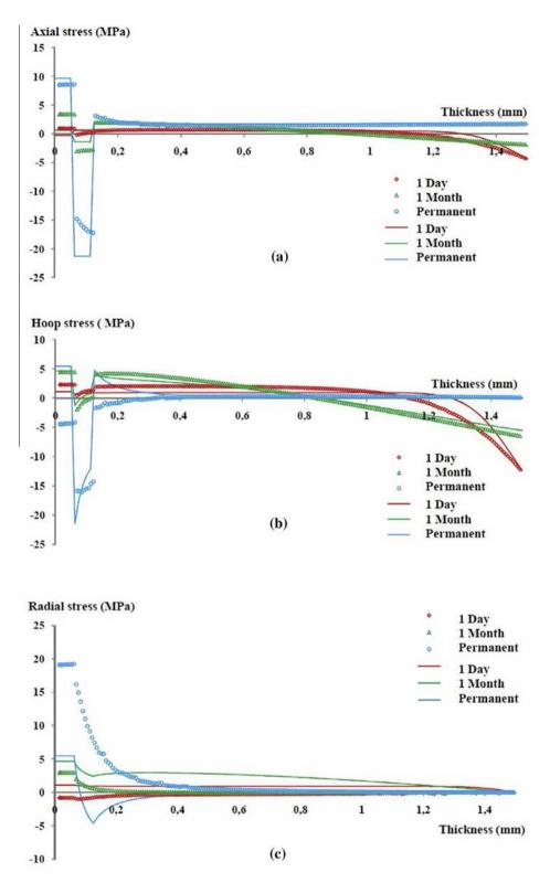
Fig. 7. Axial, hoop and radial stress in transient state obtained by finite element method (dots) and the analytical approach (lines), in the case when FBG sensor is positioned parallel to the reinforcing fibers.
