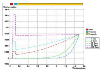
Fig. 5. Transient moisture uptake of composite sample with 22%  $v_{\rm f}$ .
