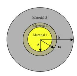
Fig. 2. Schema of the concentric cylinders model.
